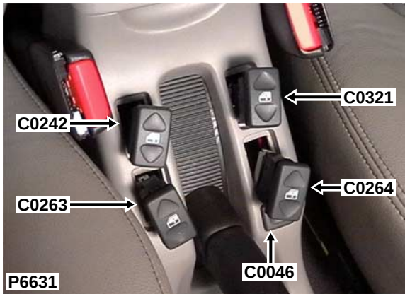
Description: Switch-Window-Front-LH Location: In rear of centre console
