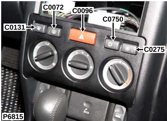
Description: Switch-Hazard warning Location: Behind centre console
